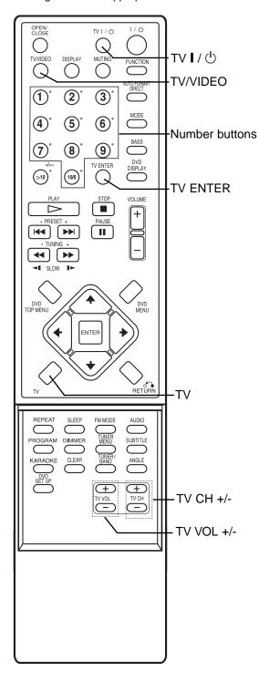
Press and hold TV I / ( ) while entering your TV's manufacturer's code (see the table) using the number buttons and press TV ENTER. Then release TV I / ( ).
